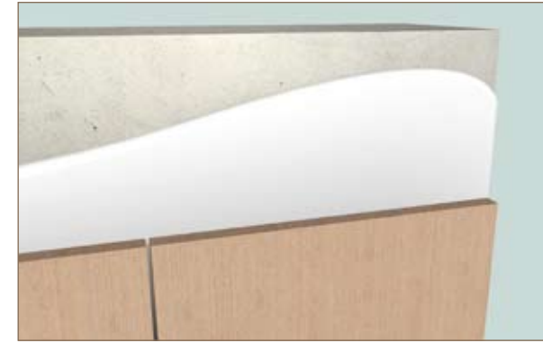
bonding on wall/plaster
